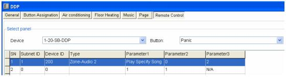
To activate the PA or Panic function, keep pressing the Panic button or PA button on G4 Remote control for 3 seconds.
